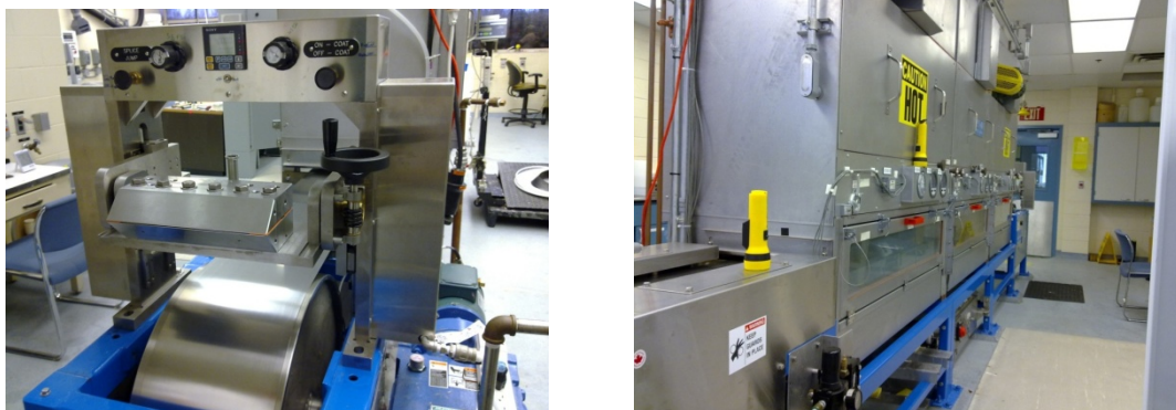
Figure 1-15. Two photographs of the FMC film-line. Left, the gel castor unit over the stainless steel belt. Right, three banks of oven through which the belt passes for drying the film.
